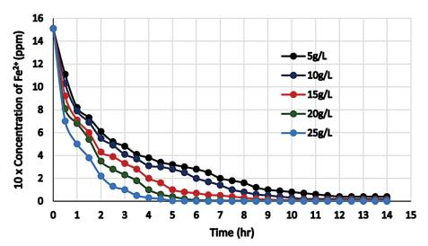
Figure 2. Concentration of Fe<sup>2+</sup> versus time at different zeolite concentrations. Zeolite mesh size 35/48
