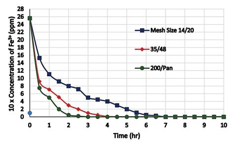
Figure 5. Concentration of  $Fe^{3+}$  versus time for different sizes of zeolite. Concentration of zeolite = 15g/L
