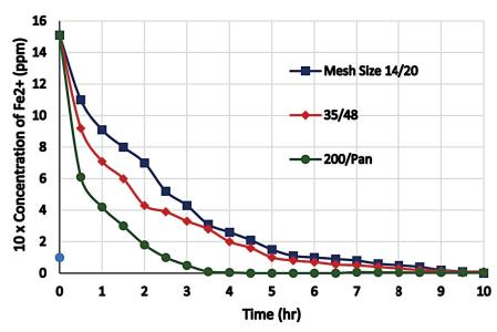
Figure 4. Concentration of  $Fe^{2+}$  versus time for different sizes of zeolite. Concentration of zeolite = 15g/L
