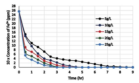
Figure 3. Concentration of Fe<sup>3+</sup> versus time at different zeolite concentrations. Zeolite size mesh 35/48
